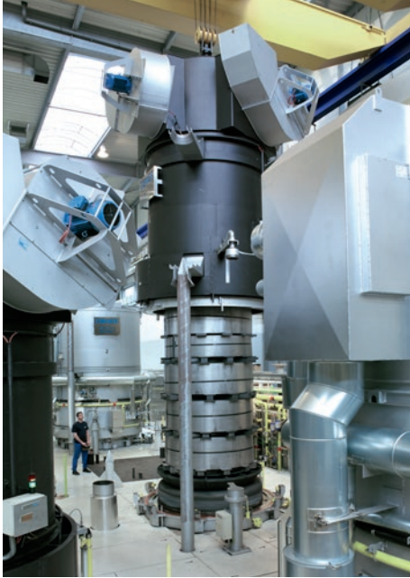
Customerspecific adaptation of standard fans in industrial furnace construction.
